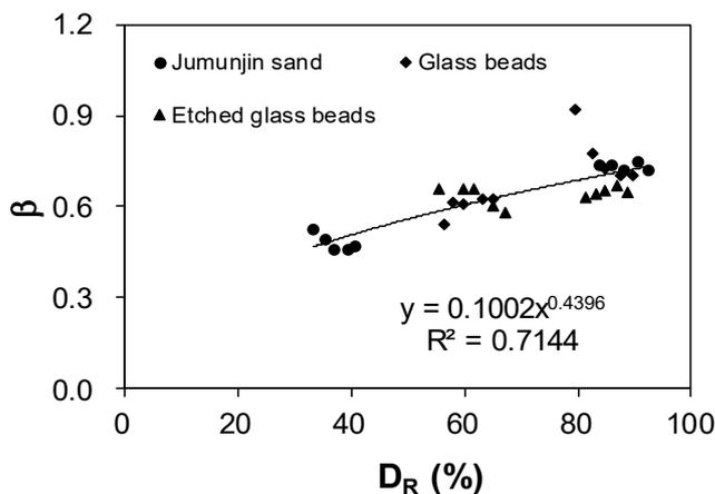
Figure 5. Values of  $\beta$  for test materials.
