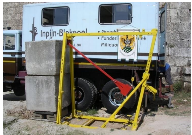
Figure 2. “Enhanced” seismic source (“Tirino Hammer”).
