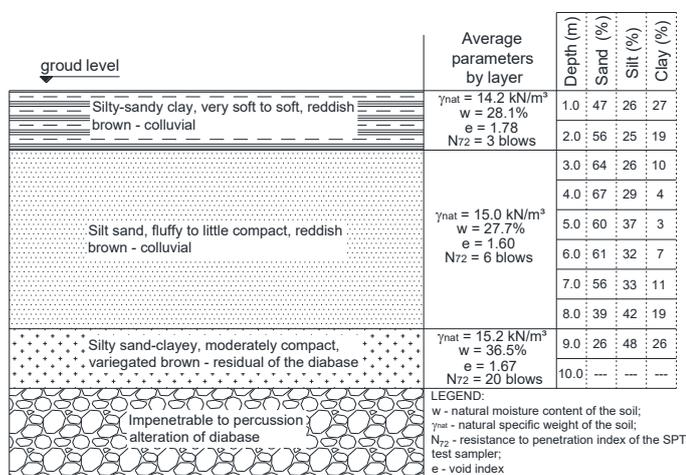
Figure 1. Simplified typical geological profile of the FEC – Unicamp Experimental Site.
