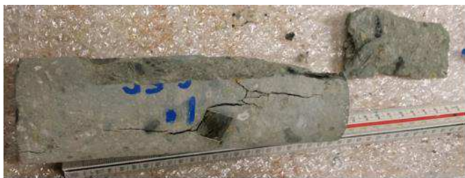
Figure 5. Failed Core Sample
