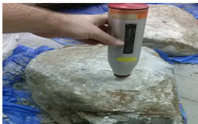
Figure 5. Sclerometry test on W4 class samples in the laboratory –(LEMETRO – UFRJ).
