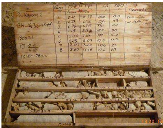
Figure 5. a sample box containing cores of a borehole in one of the tests [4].
