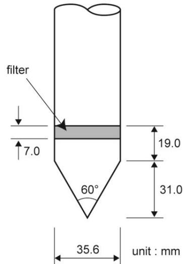
Figure 2. Dimension of the CPTU cone used in this study
