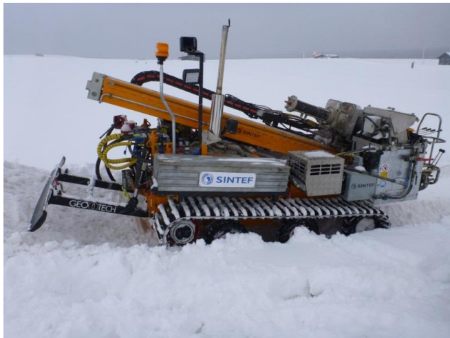
Figure 3. Geotech 504 drilling rig for Arctic condition
