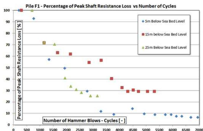
Figure 7. Percentage Shaft Loss vs No. of Cycles
