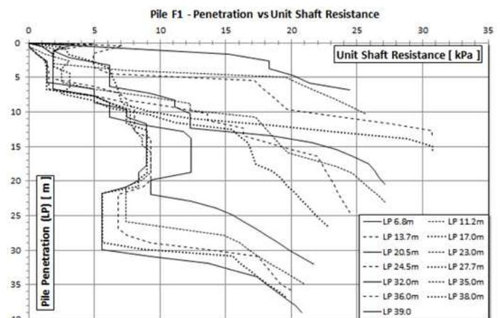
Figure 6. Shaft Resistance Values Vs Pile Penetration
