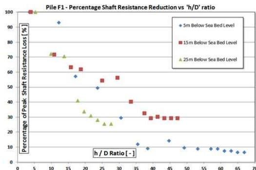
Figure 8. Percentage Shaft Loss vs h/D Ratio
