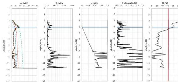
Figure 8. Pre-compaction CPT
