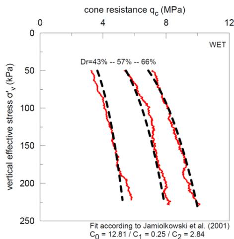
Figure 2. Results of the centrifuge CC tests on wet BAW material.
