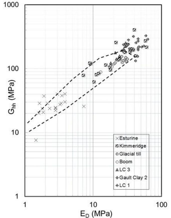
Figure 4b. Shear Modulus  $G_{hh}$  against  $E_D$
