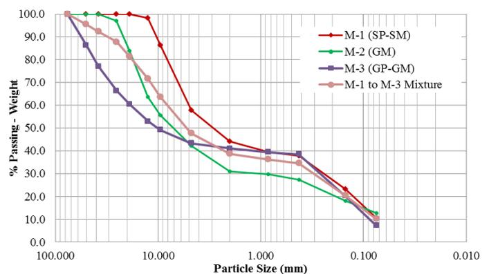
Figure 1. Grain-size distribution of angular quartz-sandstone ore material samples.
