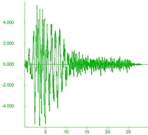
Figure 10b. Acceleration time history at the top of FLAC model  $a_x$  (m/s<sup>2</sup>) vs  $t$  (s).
