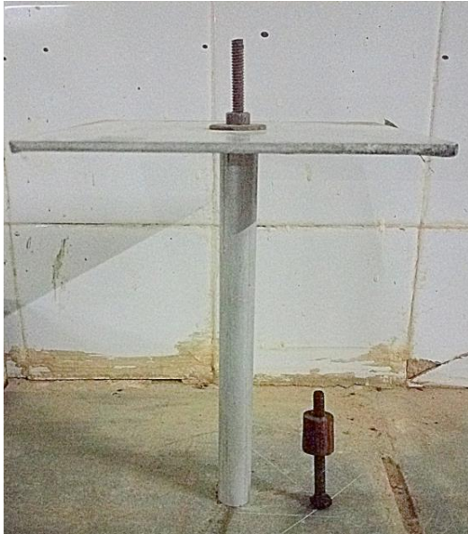
Figure 3. Connection between the pile and the raft.
