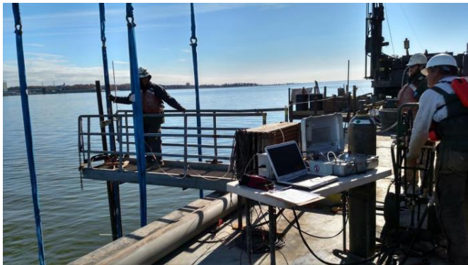
Figure 5: Typical shear wave set-up for SDMT
