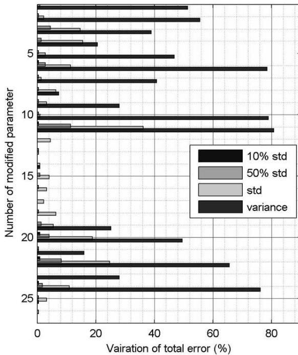
Figure 3. Results of the sensitivity analysis for the 26 original characteristics.
