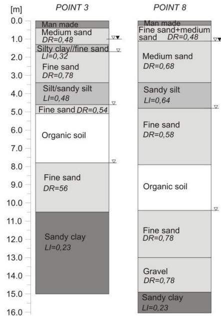
Figure 2. Example of geological profile from the test site (DR – relative density, LI – liquidity index).
