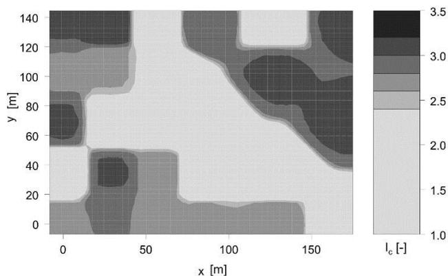
Figure 11. The 2-D interpolation model of  $I_c$  at the depth of 8,4 m.
