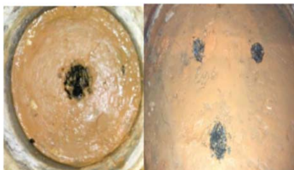
Figure 2 Installation pattern of stone column
