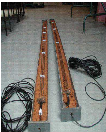
Figure 1. Photos of the basin after TDR probes installation and type of long length probes used
