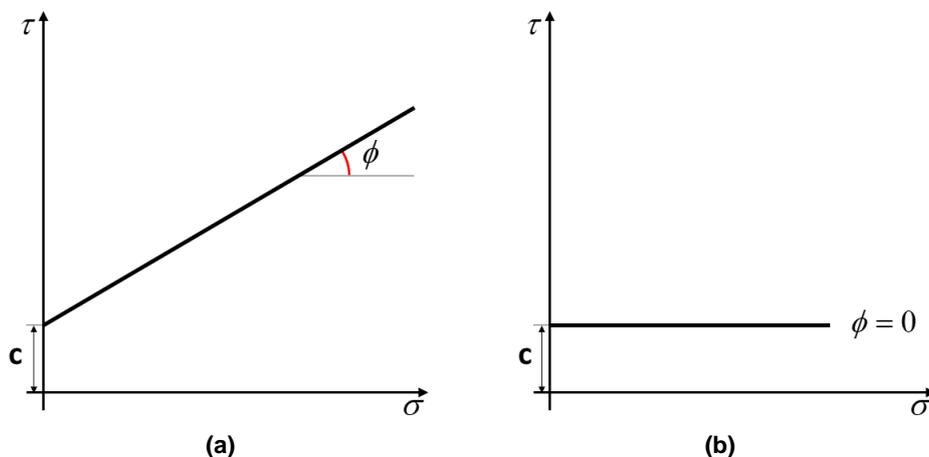
Figure 3. Relationship between normal and shear stresses for (a) a Mohr-Coulomb material, idealized in the 1950s as an "ideal sand" if  $c = 0$  and (b) a Tresca material, idealized in the 1950s as an "ideal clay"
