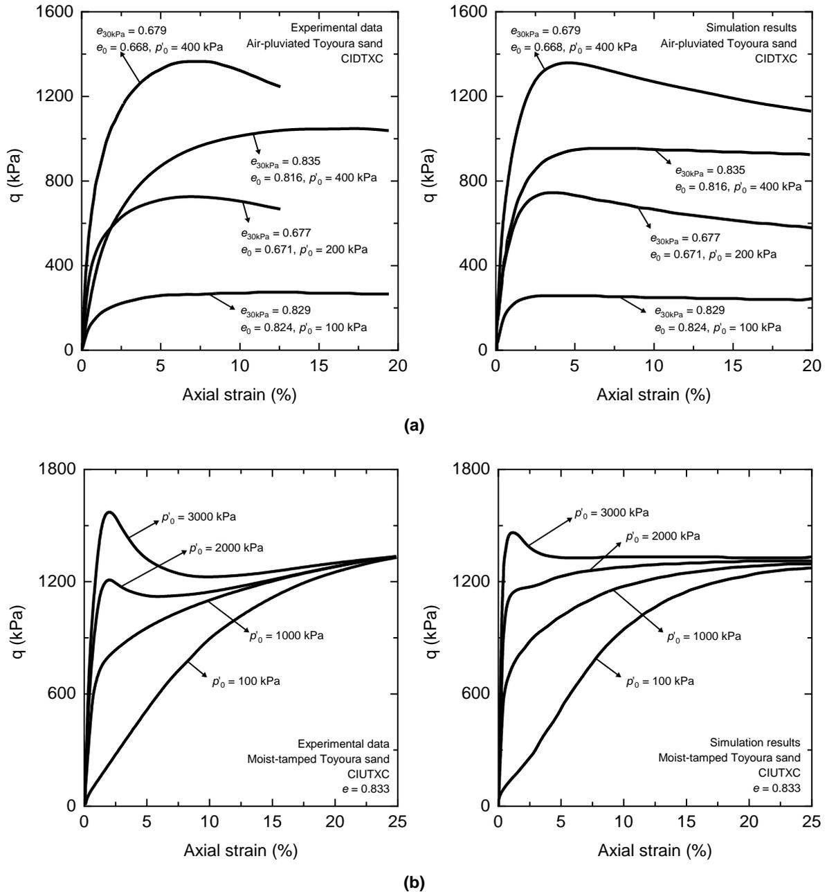
Figure 1. Results of triaxial compression test results performed on sands: (a) drained (b) undrained (Woo & Salgado, 2015)
