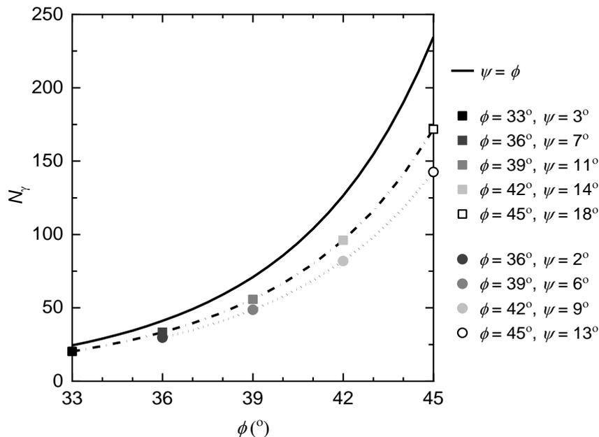
Figure 6. Comparison of values of bearing capacity factor  $N_\gamma$  calculated based on the assumption of associated flow ( $\psi = \phi$ ) with values calculated based on non-associated flow ( $\psi < \phi$ )
