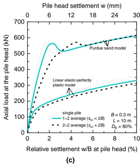
**Figure 8. Load-settlement curves obtained from analyses using: (a) a linear-elastic model; (b) a linearly elastic-perfectly plastic model with the Mohr-Coulomb yield criterion; and (c) the Purdue sand model and the linearly elastic-perfectly plastic model with the Mohr-Coulomb yield criterion (Han et al., 2019)**
