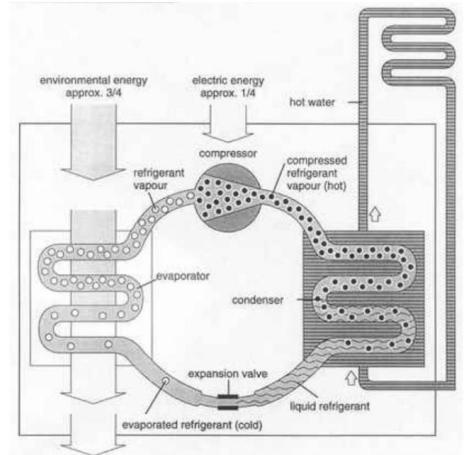
Figure 2.4 Ground source heat pump schematic, from Arup (2005)
