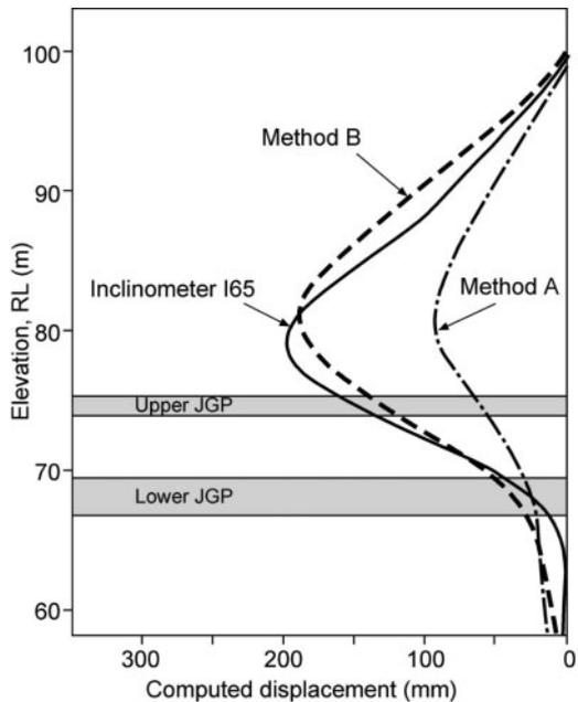
Figure 14. Maximum displacements for I65, computed and measured.
