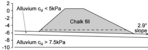
Figure 2. Embankment on very soft river muds.
