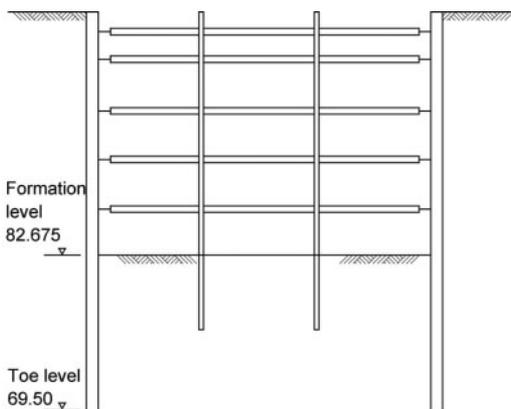
Figure 15. Deep excavation in completely weathered rock.
