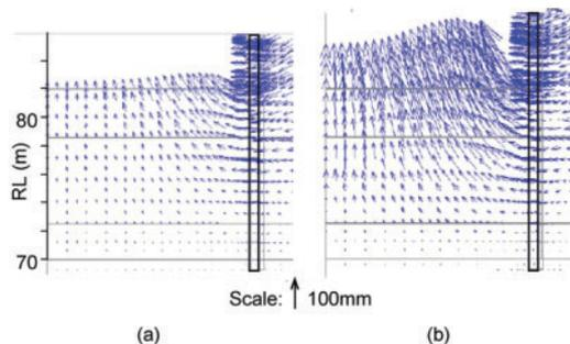
Figure 20. Ground displacements at final excavation for SSS (a)  $\psi = 0$ , (b)  $\psi = \varphi'$ .
