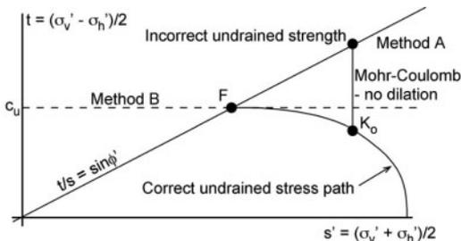
Figure 13. Modelling undrained behaviour – Methods A and B.
