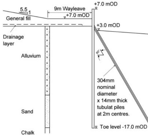
Figure 9. Sheet pile wall supported by tubular piles.
