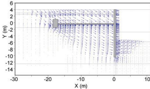
Figure 8. Failure mode shown by FE analysis.
