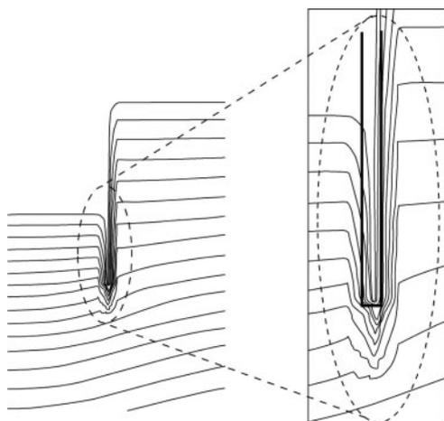
Figure 22. Impossible pore pressure contours from CRISP.
