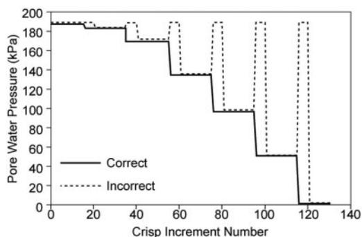
Figure 18. Computed water pressures just below final excavation surface.
