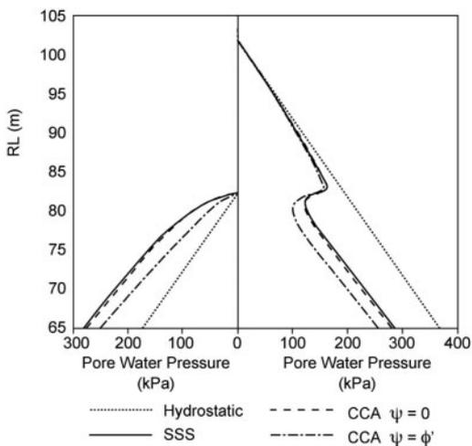
Figure 21. Computed water pressures for permeability profile B.
