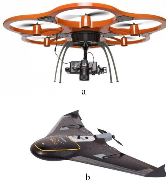
Fig. 1 a) Aibotix X6 rotary-type UAS; b) UX 5 fixed wing UAS (Leica Geosystems)
