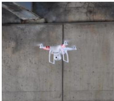
Fig. 4. DJI Phantom Vision 2 quadcopter UAS performing under-bridge inspection (Brooks et al., 2015; www.mtri.org ).
