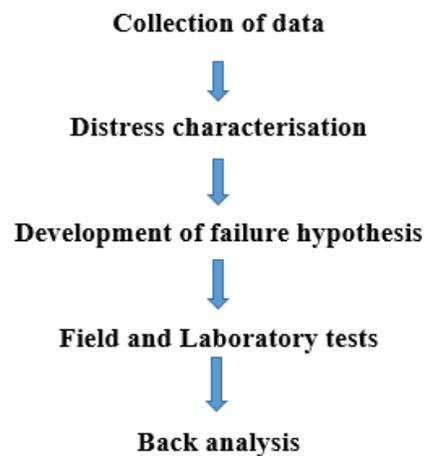
Figure 2: Different stages in failure analysis.
