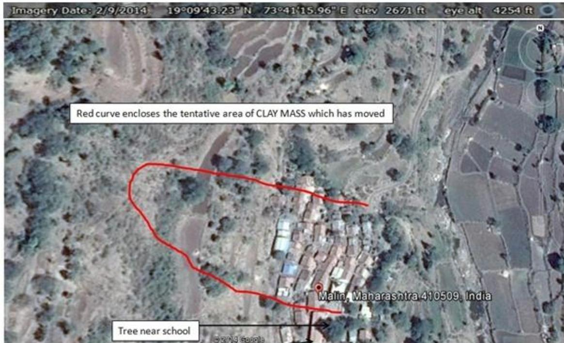
Figure 1: Landslide area
