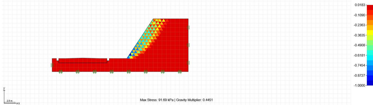
Figure 8 : Slope failure (F.O.S = 0.45)
