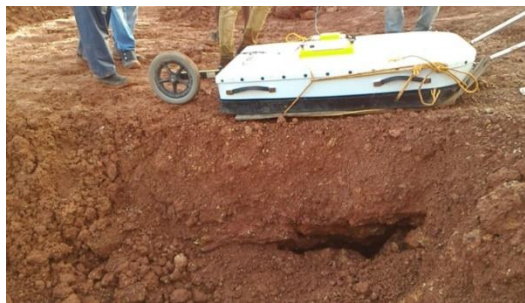
Figure 3. Survey conducted by 100 MHz ground penetrating radar over the known cavity (Location 1).
