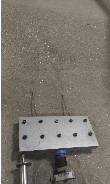
Figure 4. The photograph of the test on two L-ribs at 150 mm spacing.
