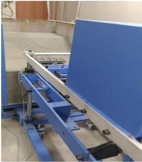
Figure 1. The pullout test set-up for rib tests
