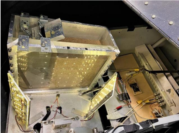
Figure 2. Model box mounted on the swing basket.
