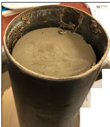
Figure 6. Cured grout sample showing a reduction in volume occurs during curing.
