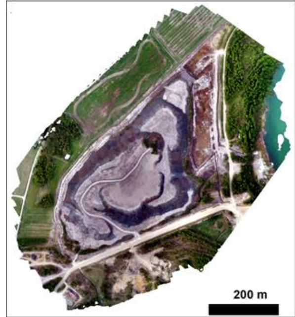
Figure 3. Orthophotomosaic of the waste rock pile generated from drone-based data.
