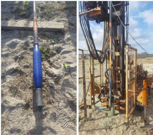
Figure 8. Preparation for in situ tests. (a) Probe assembled for the tests at Dunkirk site; (b) probe in the drill rig being positioned for the test
