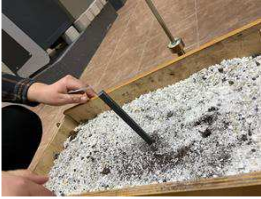
Figure 3. The process of driving the model pile into the soil in the box.
