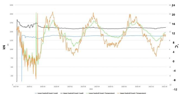
Figure 7. Measured loads with internal temperature readings for both load cells from September 2017 to summer 2021. Orange and green line shows temperature of upper and lower load cells, respectively.
