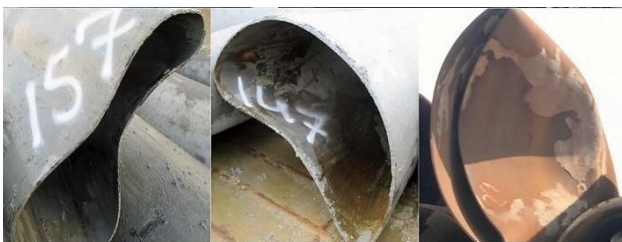
Figure 1. Extreme folding damage
