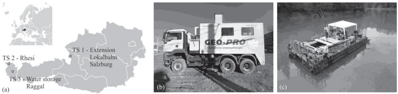
Figure 1. (a) Location of test sites TS1 - Extension Lokalbahn Salzburg, TS2 - Rhesi & TS3 - Water storage Raggal, (b) CPT-track used as penetration device at TS1 & TS2, (c) floating pontoon & CPT-fox system (Geomil equipment - Fox 2021) used as penetration device at TS3.
