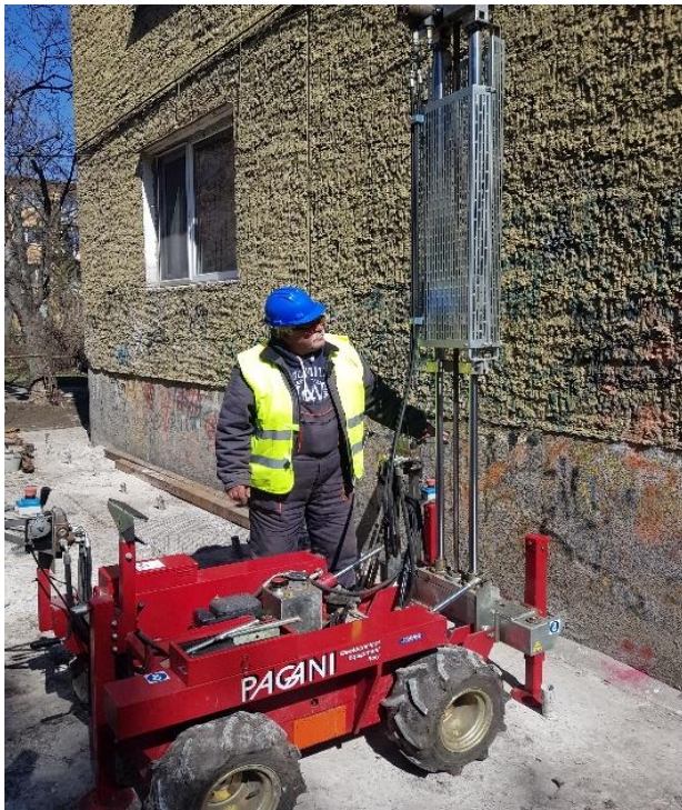
Figure 13. Dynamic penetration tests performed with a DPM (dynamic penetrometer of medium type).
