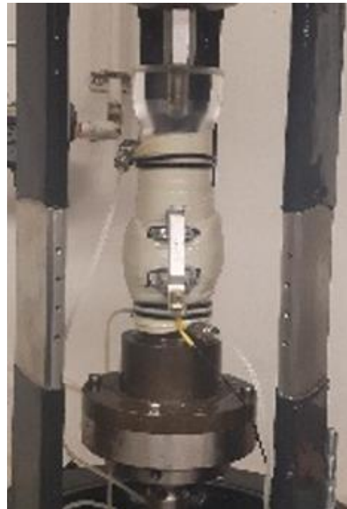
Figure 3. Hall effect local strain transducer mounted on a typical sample.
