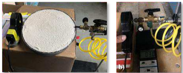
Figure 4. a) Air jet test setup set at the edge of a F60 specimen and b) taking a reading at the nozzle of the pressurized air jet with an anemometer.
