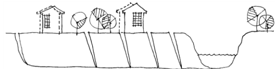
Figure 1. Schematic visualization of lateral spreading (BRANZ, 2021)
