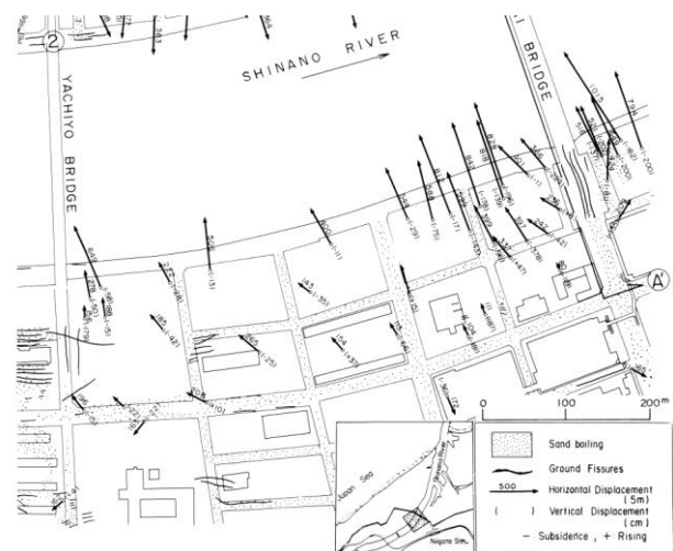
Figure 3. Permanent ground displacement vectors in the upstream area of the Shinano River after the 1964 Niigata earthquake (from: Hamada and O'Rourke (1992))
