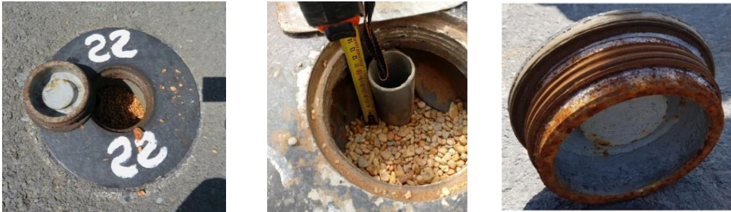
Figure 4. Details of a sand tell-tales device.
