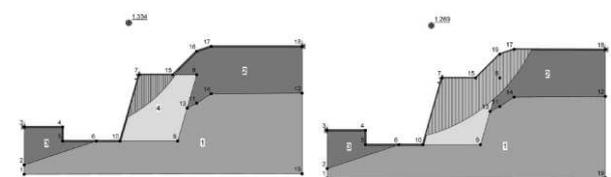
Figure 3. Critical slip surfaces in static and seismic conditions.
