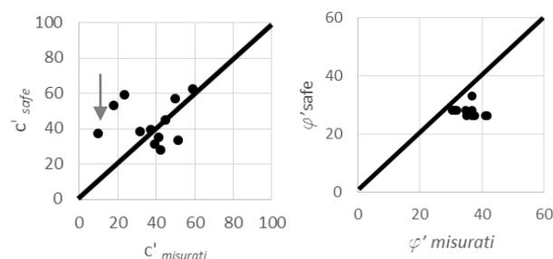
Figure 2. Quicklime treatment: calculated versus measured values of shear strength parameters.
