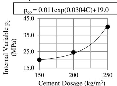
Figure 2. Initial value for the internal variable  $p_c$ , as a function of the cement dosage, C ( $R^2 = 0.9952$ ).
