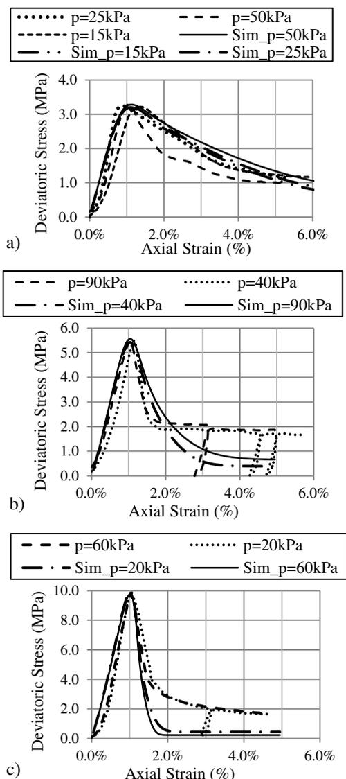
Figure 1. Simulations vs experimental data – deviatoric stress vs axial strain: a) 150 kg/m<sup>3</sup>; b) 200 kg/m<sup>3</sup>; c) 250 kg/m<sup>3</sup>.
