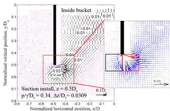
Figure 1. Incremental soil displacement vectors at the bucket penetration of  $z/D_c = 0.5$  with  $\Delta z/D_c = 0.03$ .
