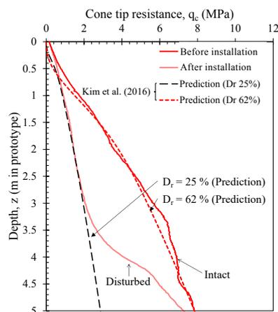
Figure 3. Results of cone penetration test at locations inside (disturbed soil) and outside (intact soil) the bucket.
