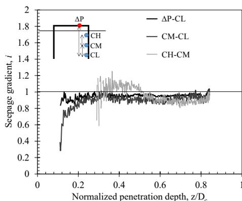
Figure 2. Seepage gradient along the inner bucket wall during suction installation.
