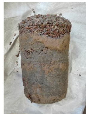
Figure 2. The vertical reinforcing drain element pulled out of the soil after 56 days.
