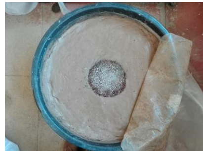
Figure 1. The vertical reinforcing drain element from dry concrete mix installed into soft water-saturated clayey sand.
