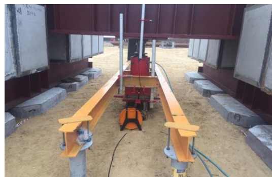
Figure 2. Testing platform for static compression load test
