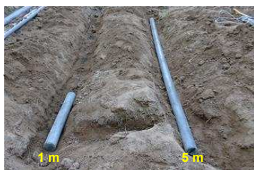
Figure 2. Soil nails of lengths of 1 m and 5 m.
