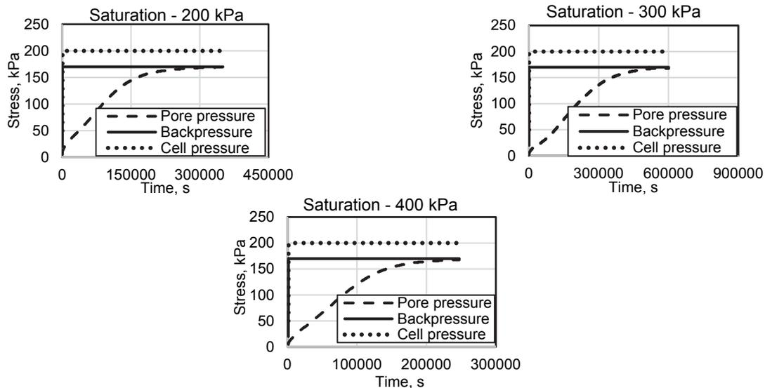
Fig. 5. Specimen saturation by increasing back pressure (SCD method)
