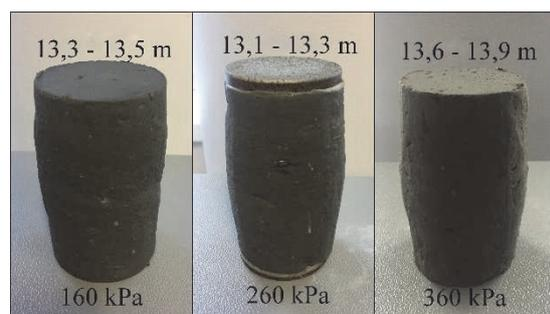
Fig. 4. Samples after UCU tests
