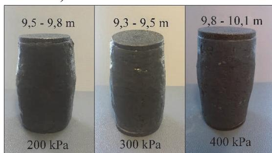
Fig. 3. Samples after SCD tests
