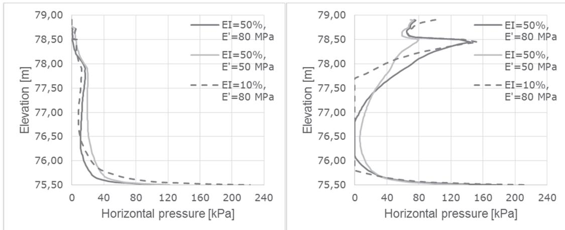
**Fig. 4:** SLS horizontal pressures acting on the gallery wall. Left: Pressure before forced displacement. Right: Total horizontal pressure after 10 mm forced horizontal displacement of the large concrete base slab.
