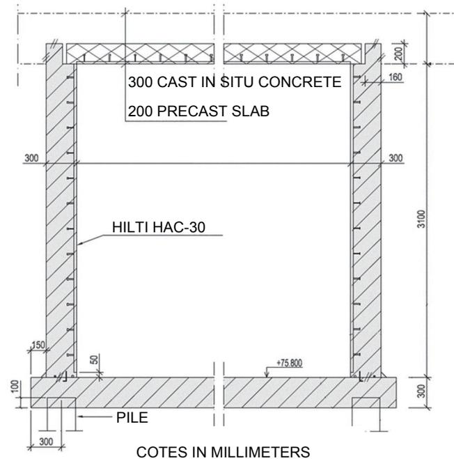
**Fig. 2:** Typical detailed cross-section of the installation gallery structure
