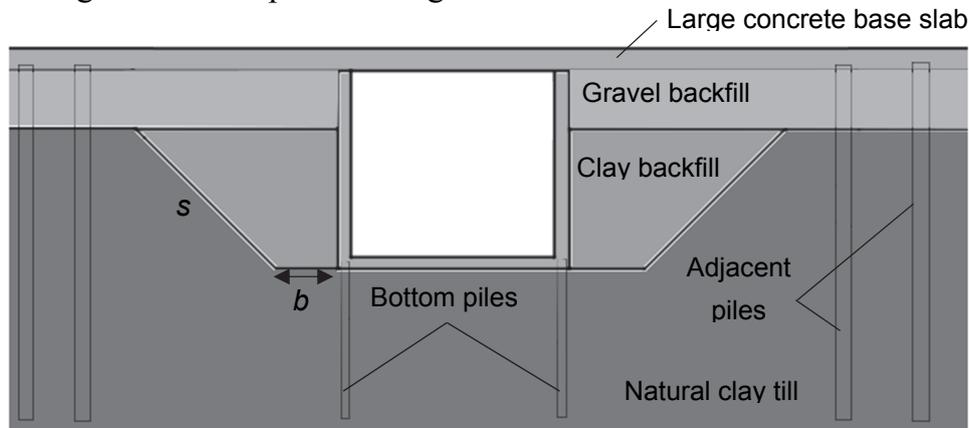
**Fig. 1:** Conceptual sketch of the installation galleries under D01 and D03
