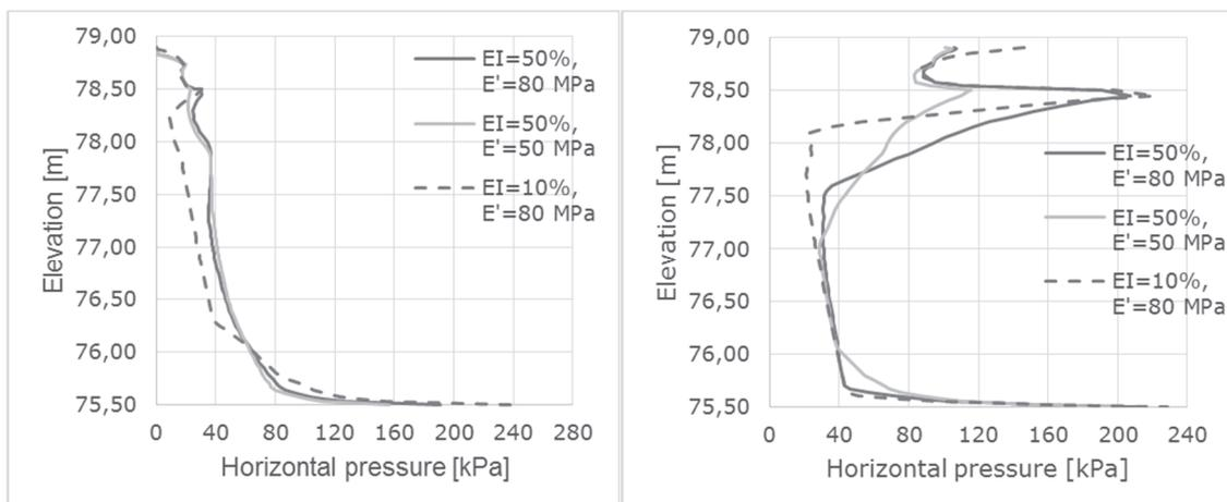
**Fig. 5:** ULS horizontal pressures acting on the gallery wall. Left: Pressures after raise of ground water level. Right: Pressures after 10 mm forced horizontal displacement of the large concrete base slab.
