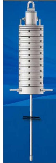
Figure 2: Sketch of the Deep-sea GraviProbe.
