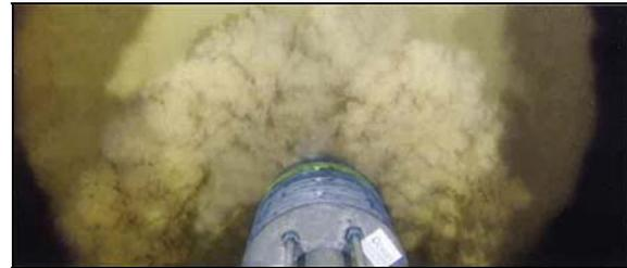
Figure 8: Impact of the wider GraviProbe body at the seabed, after 4 m penetration of the shaft & cone. Notice the perfectly straight alignment during penetration.
