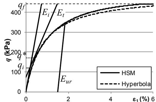
Figure 3. Triaxial test - HSM and hyperbola
