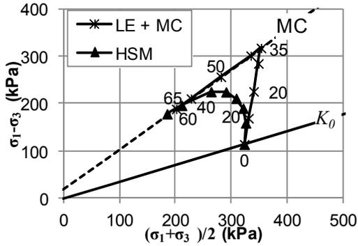
Figure 4. Stress path at the sidewall
