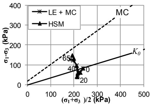
Figure 5. Stress path near the crown
