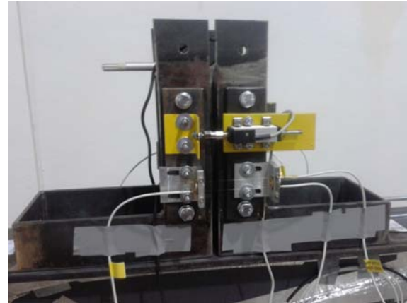
Figure 14. L-consoles with displacement transducer and tested optical FBG fibres
